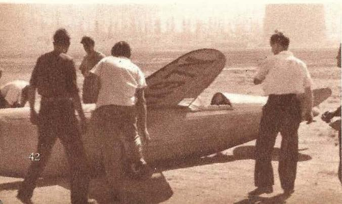
**A** RACING plane with a wing span of only 12 feet has been designed and built by Tom Floyd of California. Due to its tiny span, the speedster, which has been named the *Floyd Bean Special* after Floyd and his pilot, Bob Bean, has a landing speed of 120 miles an hour.
