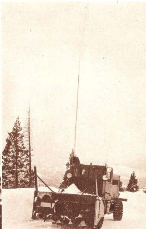
Left: Radio equipment is conveniently located in front of plow operator. Above: Plow with radio antenna raised works in isolated mountain sector. Below: The foreman transmits instructions to a plow operator.
