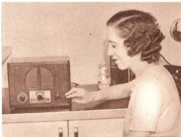
Above: This is "central" of the house communications system. Resembling a small radio receiver, the amplifier rests on a kitchen surface. From here one may speak to almost any other part of the house. Right: Another convenience is the electric blanket with its control box located on a convenient stand. Above the control box is a speaker-microphone unit of the communications system.
