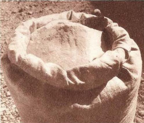
Casein appears in the form shown in the photo at left before it undergoes a dissolving process with chemical reagents.
